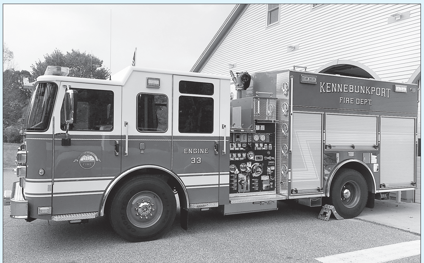
Engine 33, our newest apparatus, is a 2017 Pierce Saber pumper that has been assigned to help protect Goose Rocks Beach. It carries 1,000 gallons of water, 2,000 ft of four-inch hose, and a 1,250 gpm pump, along with state-of-the-art gas detection and thermal imaging equipment.
