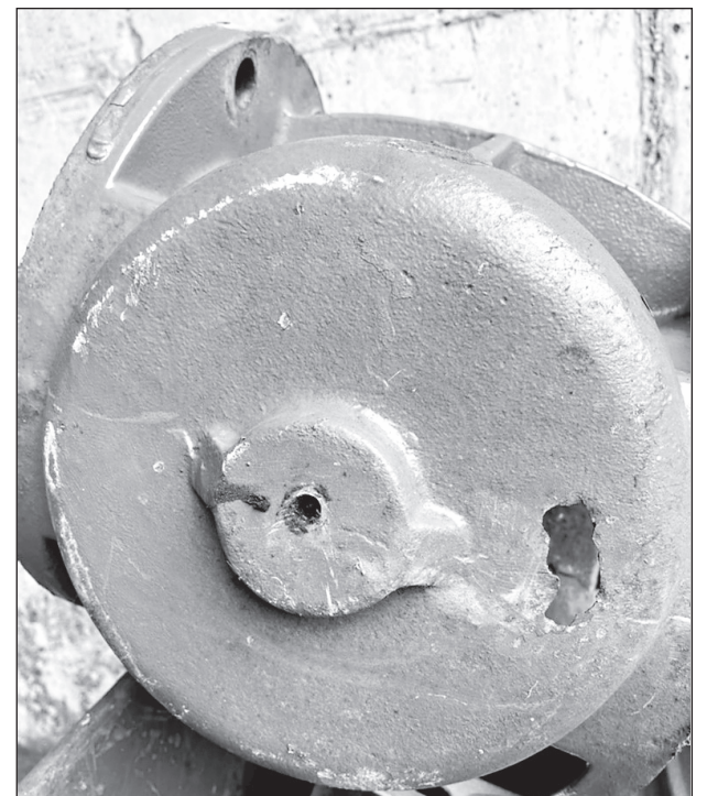
Picture of rotted gate valve from Wildes District Pump Station resulting in $11,000 emergency repair. See hole in bottom right-hand side of casting.
