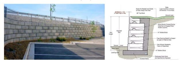
Figure 2-3: Vertical Retaining Wall Example and Typical Schematic Detail. Detail Courtesy of Redi Rock
