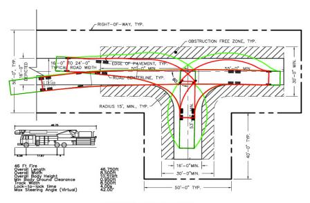
HAMMERHEAD TURNAROUND DETAIL SCALE: 1"=20'
