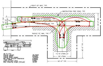
HAMMERHEAD TURNAROUND DETAIL SCALE: 1"=20'
