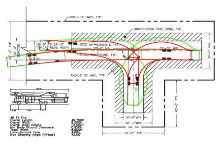
HAMMERHEAD TURNAROUND DETAIL SCALE: 1"=20'
